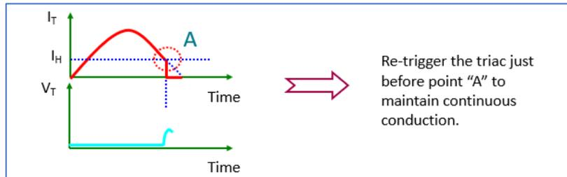
Fig. 25 Graphic showing interaction of  $I_T$  and  $I_H$
