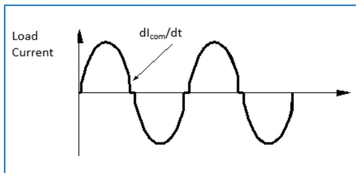
Fig. 33  $di_{com}/dt$  illustration for a rectifier fed inductive load
