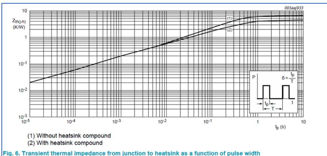
Fig. 6. Transient thermal impedance from junction to heatsink as a function of pulse width
