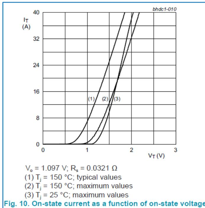
Fig. 27 Example of static characteristic  $V_T$  and graphic
