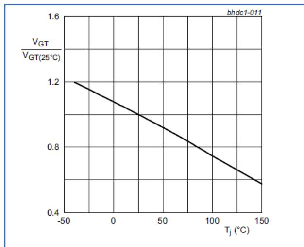
Fig. 26 Normalized  $V_{GT}$  versus junction temperature
