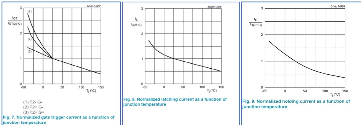
Fig. 23  $I_{GT}, I_L$  and  $I_H$  temperature dependency graphics (BTA312-800CT)
