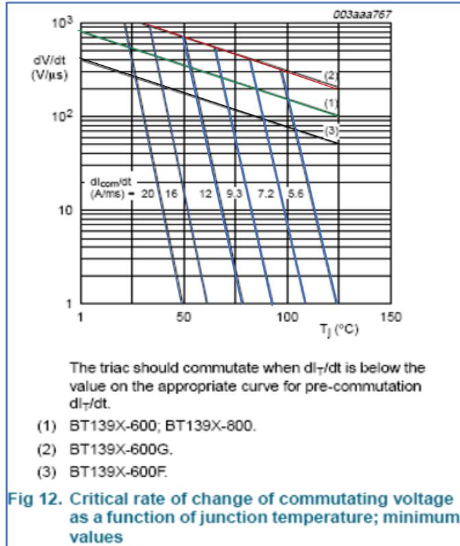
Fig. 35 Illustration of interdependent relationship between  $di_{com}/dt$ ,  $dV_{com}/dt$  and  $T_j$
