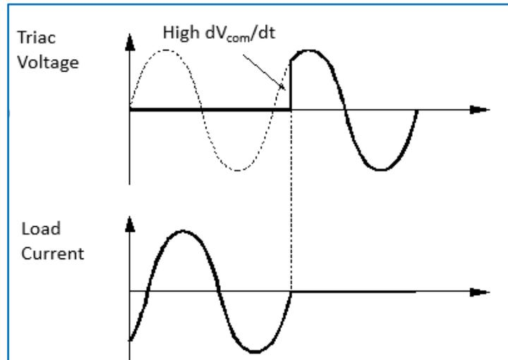
Fig. 34  $dV_{com}/dt$  illustration for an inductive load
