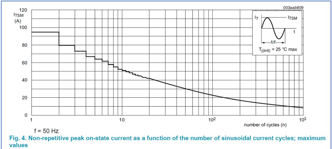
**Fig. 12 Example of  $I_{TSM}$  versus number of pulses**
