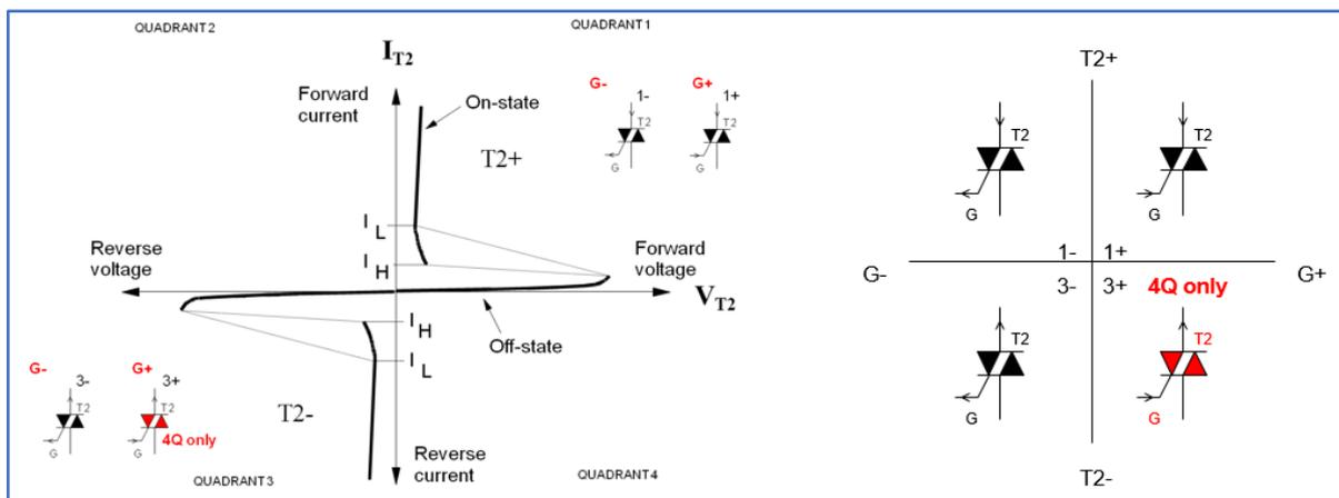
Fig. 20 Triac operating characteristic and triggering options
