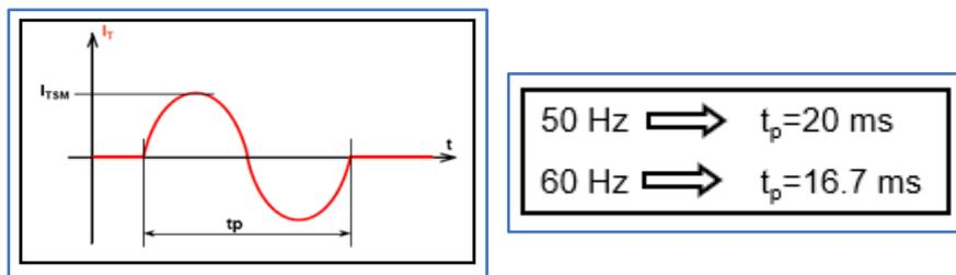
Fig. 10 Example of non-repetitive peak on state current rating
