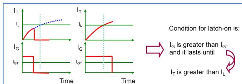
Fig. 24 Graphic showing interaction of  $I_{GT}$  and  $I_L$
