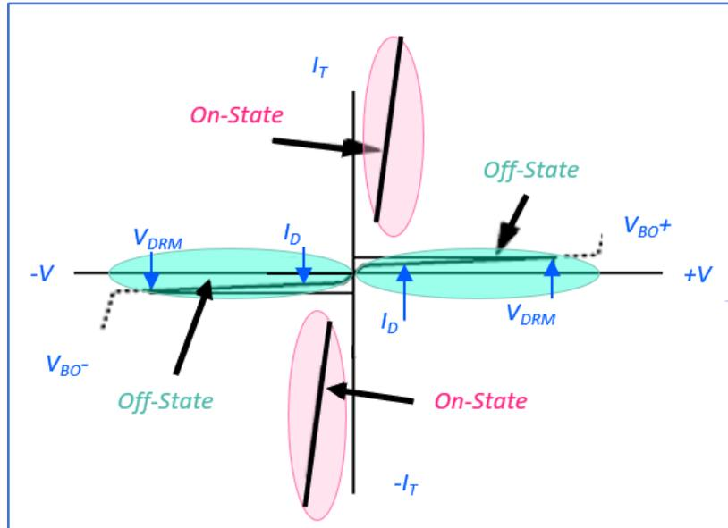
Fig. 6 Blocking off-state voltage and on-state conduction operating regions
