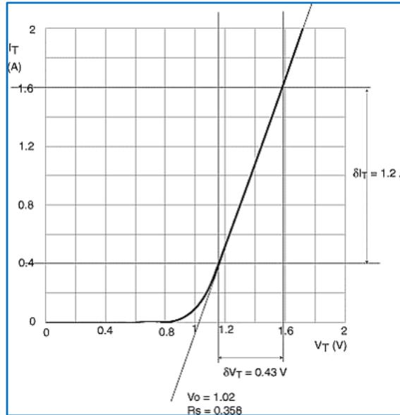
Fig. 28 Example graphic showing  $V_0$  and  $R_s$  derivation
