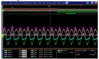
Figure 3: WeEn SCR: typical waveform used in UPS rectifier circuit (Purple: SCR1 A-K current; Yellow: SCR1 A-K voltage ; Green: AC mains current ; Blue: SCR2 A-K voltage)
